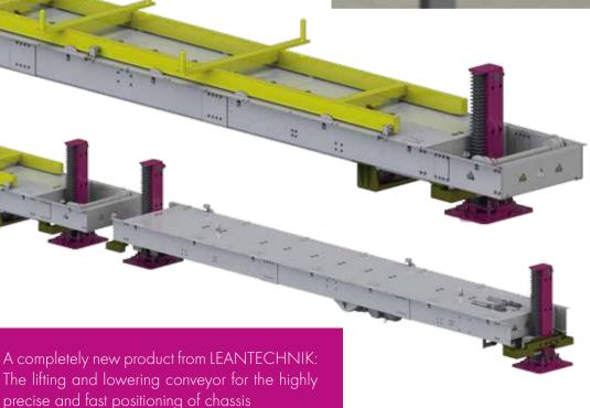
Our newest product for the automotive industry is the lifting and lowering conveyor, which we developed. The lifting and lowering conveyor is composed of hub gear elements, a motor, a steel structure and a skid conveyor and ensures the precise transfer of chassis between two points on the assembly line. The system lowers, lifts and conveys heavy loads in a matter of seconds. Two synchronized lifting columns bring the transport frames to the required position precisely at the time scheduled.
